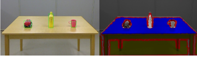
Fig. 3: Examples of the used objects and the corresponding 3D point cloud information: (A) car, (B) bottle, and (C) cup.
